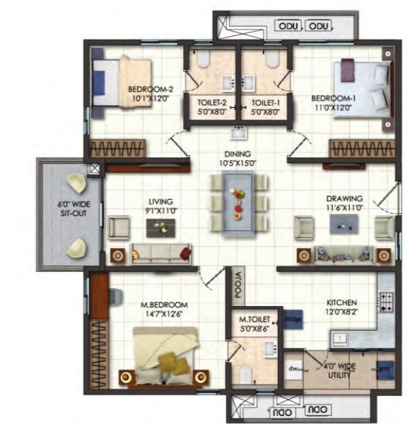
Carpet Area 1128 Sft I Wall Area 88 Sft Balcony & Utility Area 127 Sft I Common Area 372 Sft
